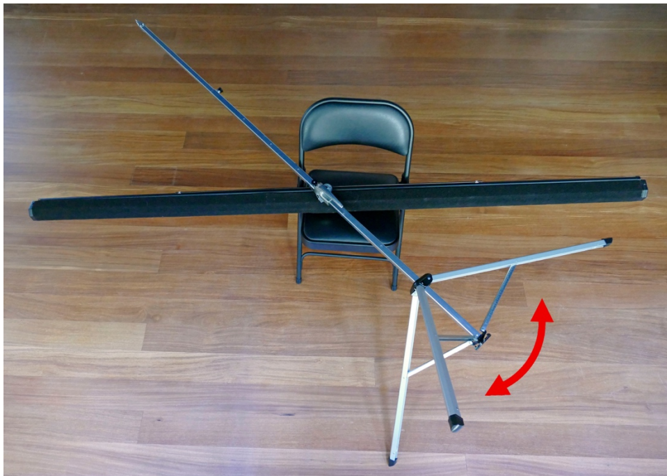
Opening the tripod legs
