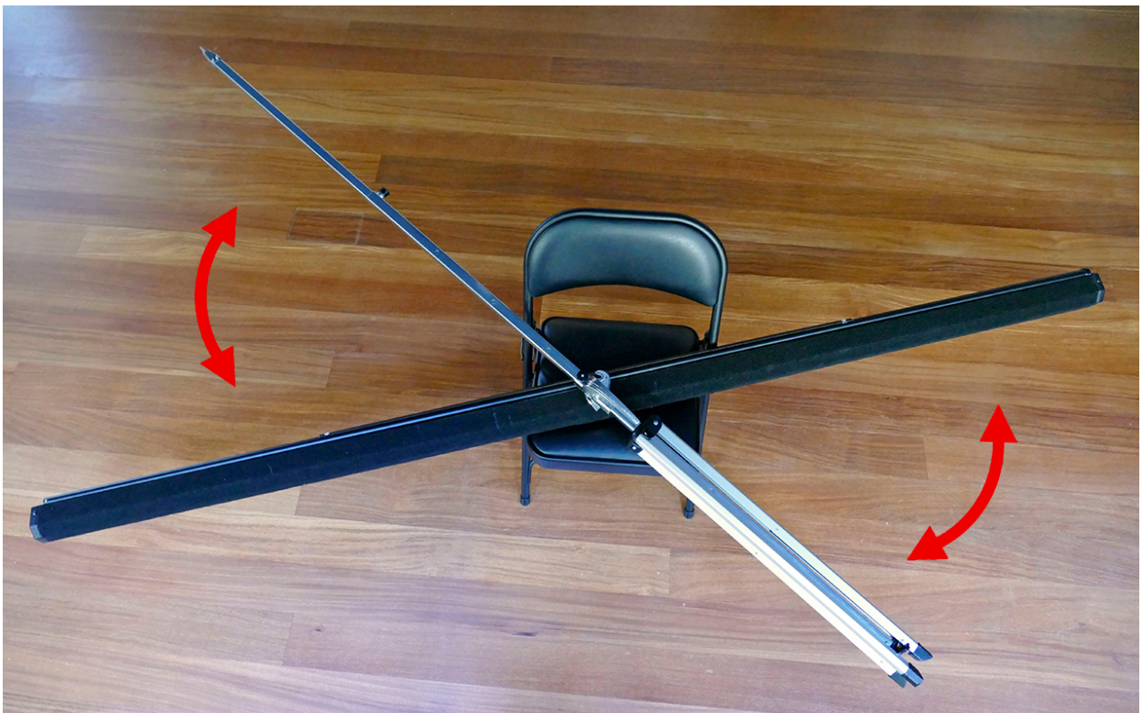
Canvas orientation before opening tripod legs
